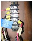
The electrical wiring to the mast lights was in good condition. I had previously installed a terminal block for the connections and each wire had been tagged with a label. This was a big help.
