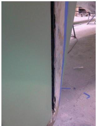
The rudder support needed patching. Vinyl ester resin putty with adhesive filler was used to fill in the small voids.
