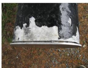
A steel plate had been concreted into the keel below the mast step. The plate was tapped for two 3/8" by 2" bolts. The threads were fine. There was a small, 1/8" thick, rubber pad between the step and the keel. It was in reasonably good condition; so it was returned to insulate the mast step and keel plate metals. The new aluminum mast base plate would be affixed to the restored concrete encased keel plate by means of the original stainless steel bolts.
